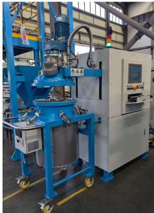
Portable mixer is consists of vacuum pump, mixer lid, lifting device, steel frame and control cabinet.
